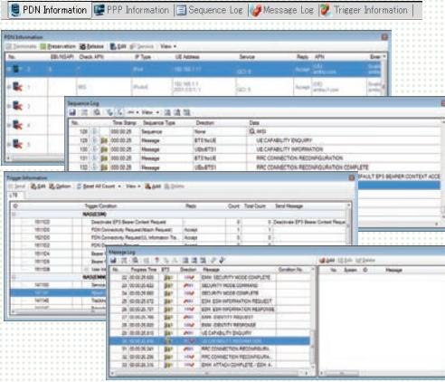
**5** Both base station parameters and packet communications can be controlled. Changes to status change parameters during testing are reflected immediately on-screen.
